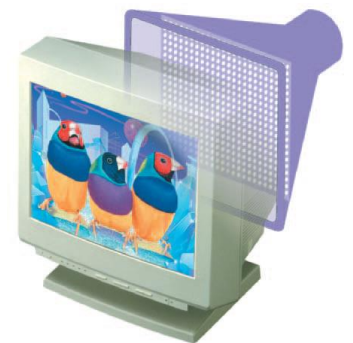
Figure 2.23: CRT screen coated with tiny phosphor dots
