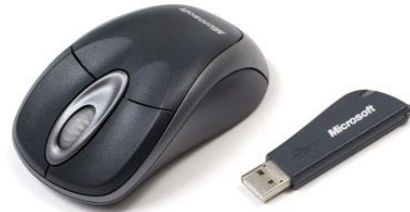
Figure 2.6: Wireless mouse with Bluetooth dongle
