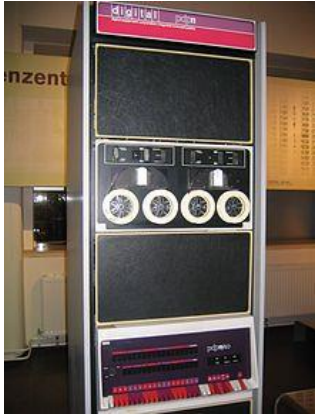
Figure 1.4: A PDP-11, model 40, an early member of DEC's 16-bit minicomputer family, on display at the Vienna Technical Museum
