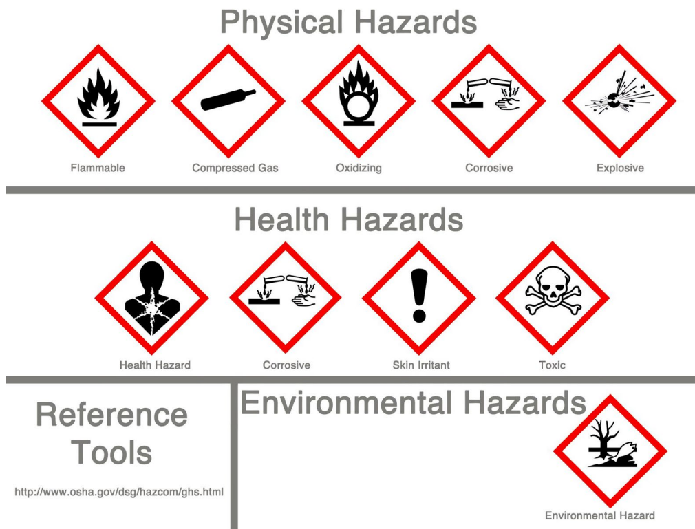
Fig. 15: some example of health hazards
