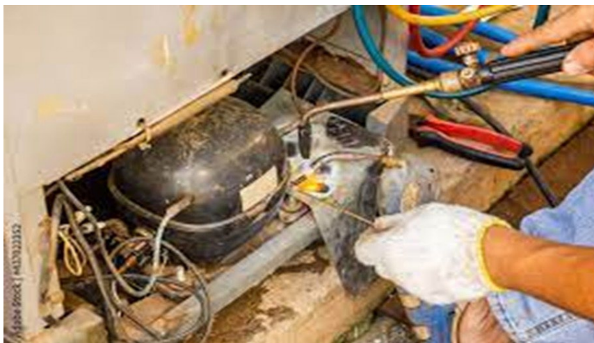
Fig. 5.15: Repair and maintenance with gas welding.
